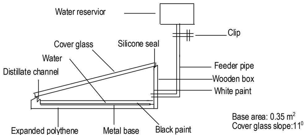
**Figure 1:** Cross-section of the solar still.
