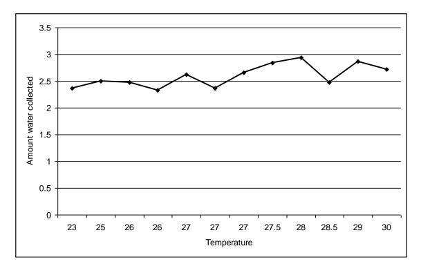
Figure 3. Amount of water [L/m²/day] collected in the Lowveld at different ambient temperatures [°C]
