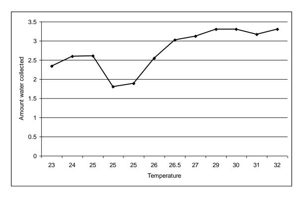
Figure 2. Amount of water [L/m²/day] collected in the Middleveld at different ambient temperatures [°C]
