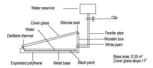
Figure 1: Cross-section of the solar still.
